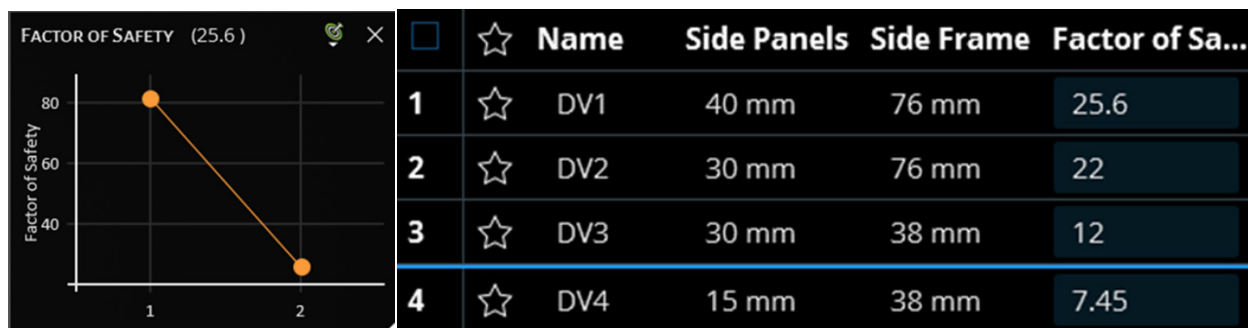
Figure 12: Structural Simulation Parametrization Results
